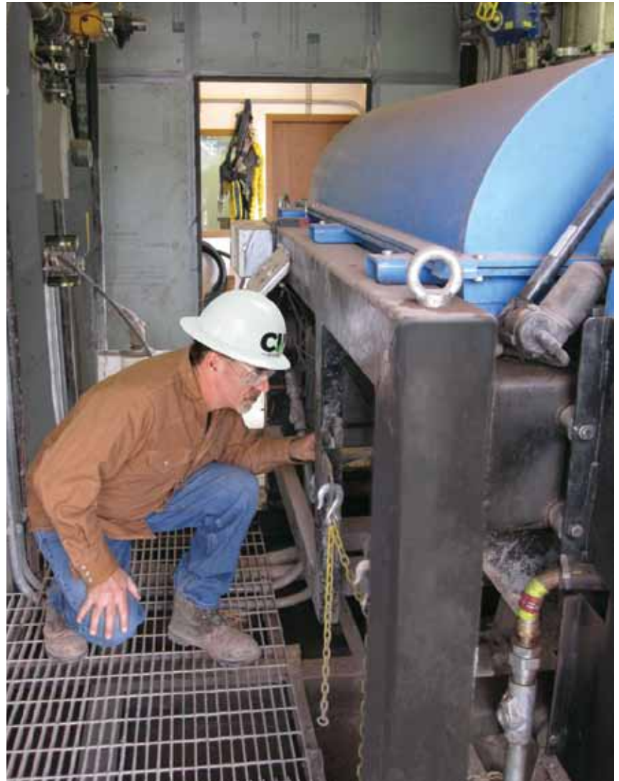
CRS continually monitors results to ensure quality. A technician checks a centrifuge that minimizes solids to meet customers' specifications.
