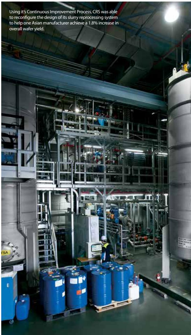
Using its Continuous Improvement Process, CRS was able to reconfigure the design of its slurry reprocessing system to help one Asian manufacturer achieve a 1.8% increase in overall wafer yield.
