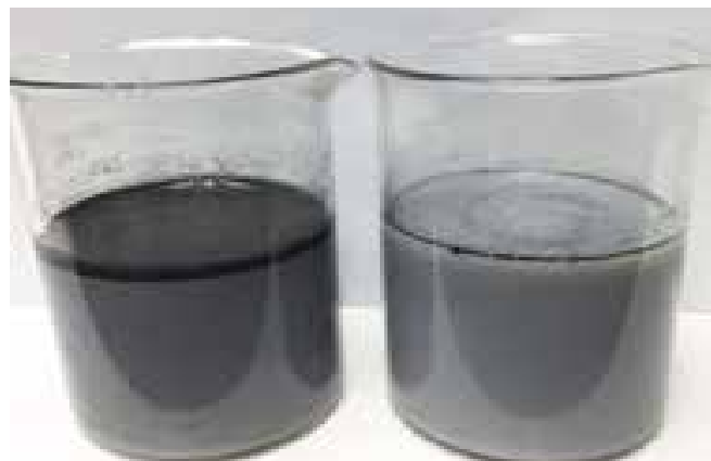
Left: Hot Mill Active System Right: TUF-D Permeate
