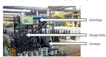
To ensure a high quality level of emulsion available to the manufacturing process, CRS designed a custom process flow to separate AWPE's salt water tank and emulsified fluids before centrifugation.
