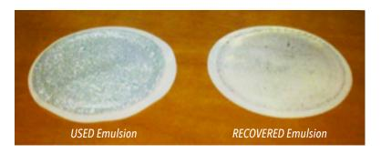
The particulate filter load test shows that approximately 95% of particles larger than 10µm are being removed.
